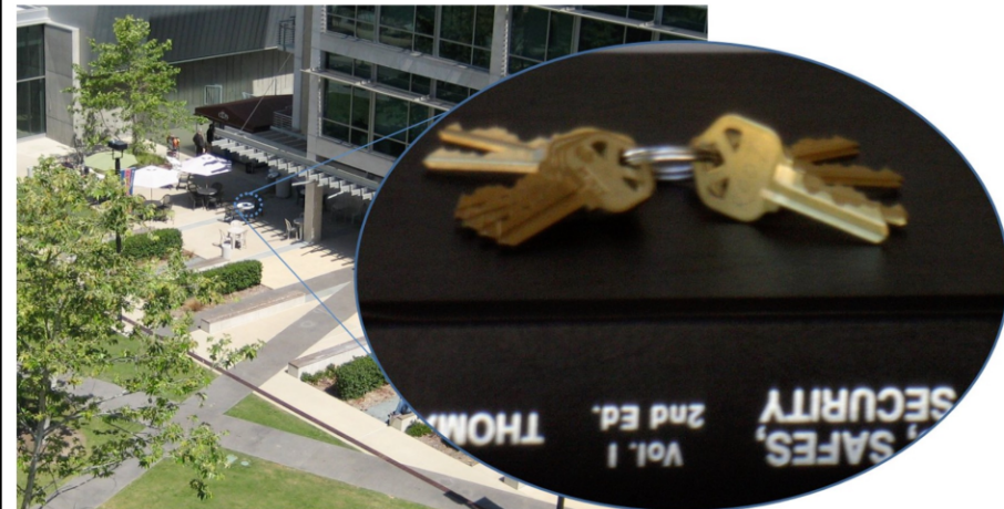
Figure 9: Our proof-of-concept telephoto experiment. The key image, captured at a distance of 195 feet, was correctly decoded as 74753.
