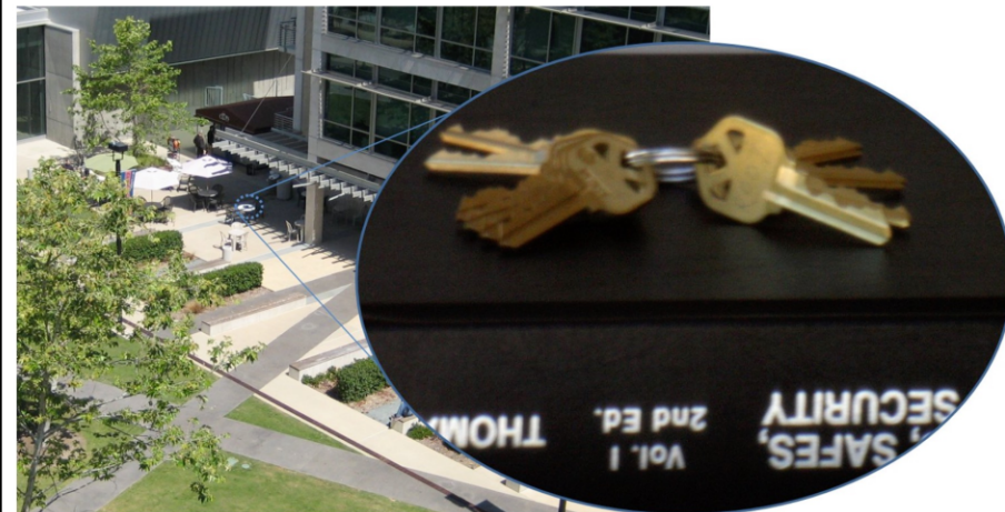
Figure 9: Our proof-of-concept telephoto experiment. The key image, captured at a distance of 195 feet, was correctly decoded as 74753.
