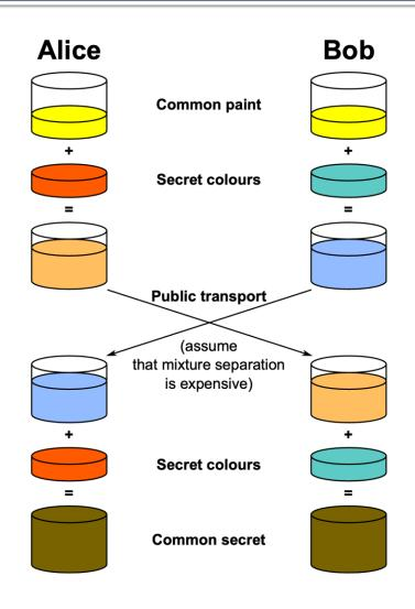
The **Diffie-Hellman Key Exchange** is a construction through which two parties can safely create a shared secret in the presence of a passive attacker.
